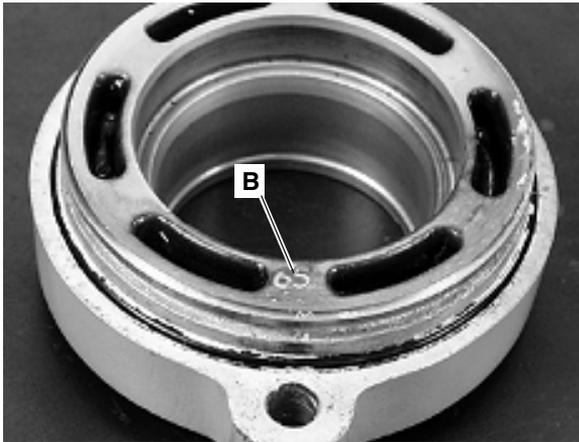
**32.** There is a dimension (**B**) punched on the rear bearing housing. This dimension is stamped underneath the bearing housing, and varies between 50–70. In this case, the distance is 65 mm (2.5591").
