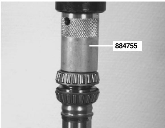
16. Install the other roller bearing inverted, i.e. with the smaller end upwards. Use mandrel **884755**.
