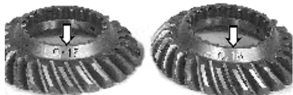
**16.** Measure the clearance between the flange on both sides. Use a feeler gauge.
