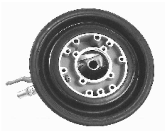
**63.** Put the rubber sleeve on the upper gear housing.
