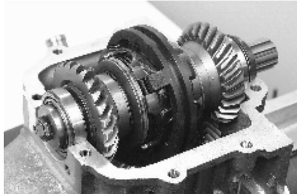
3. Lift the input shaft out and remove the seal ring, the outer bearing races and the shims on both sides. Scrap the seal ring.
