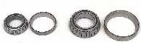
56. Check the bearing and bearing races for wear.
