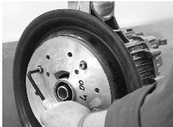
4. Remove the adapter plate and remove the rubber sleeve.
