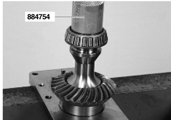
22. Install the inner roller bearing with tool no. **884754**.
