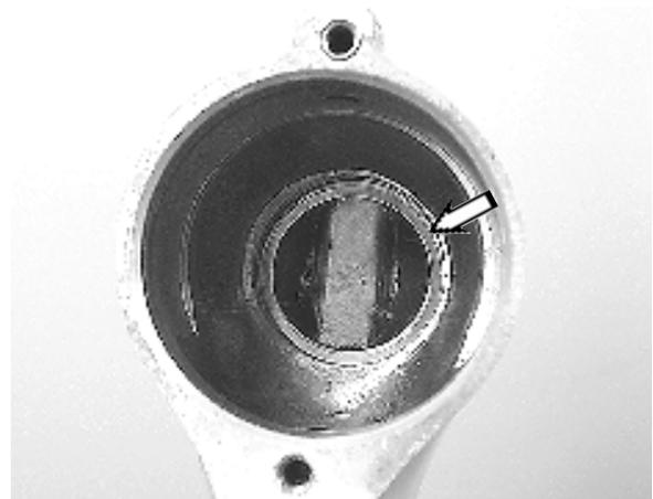
27. Put shims of the correct thickness in the lower gear housing. Add a further 0.05–0.10 mm (0.001968–0.003936"). In this case, we put a total of 1.00 mm (0.03937") shims in the housing.
