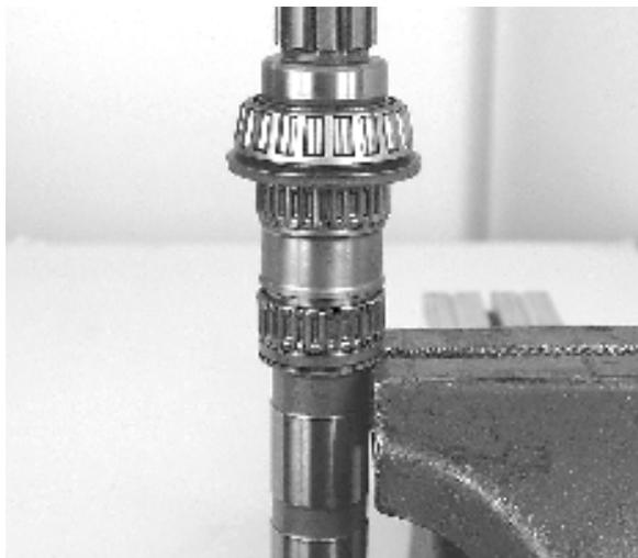
6. The bearing – sintered washer – needle roller bearing – spacer – needle roller bearing – spacer – shim and key are left on the shaft.
