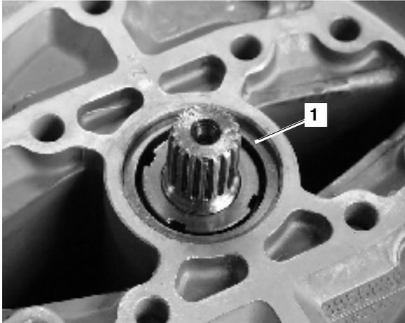
58. Check that there is no end float in the vertical shaft. Then install spacer ring (1).
