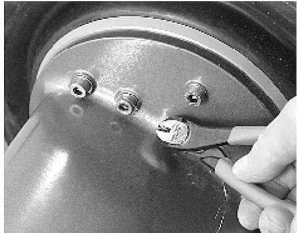
**68.** Secure four of the screws, the ones with holes in their heads, with locking wire, two screws on each side as in the illustration.
