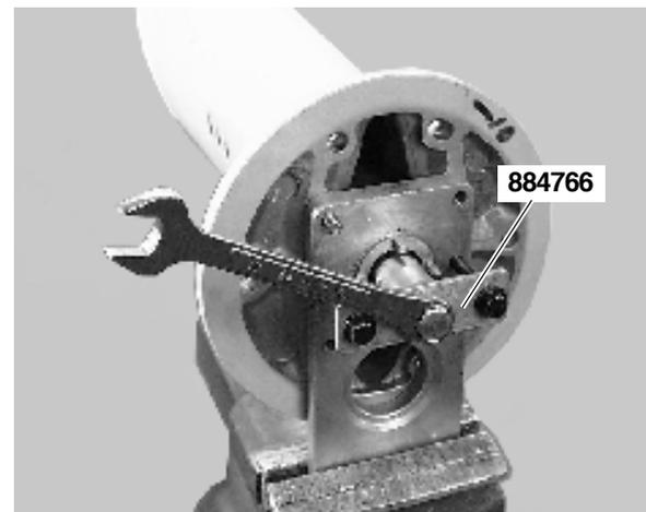
**50.** Install the propeller shaft again and turn it round in both directions. Brake the propeller shaft strongly.
