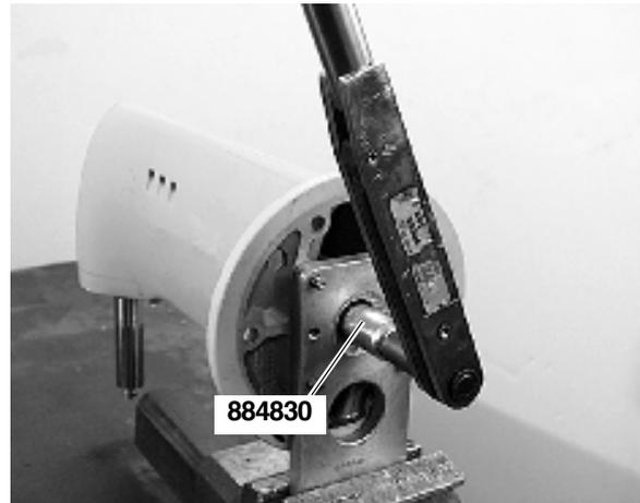
47. Install tool **884830** on the vertical shaft. Turn the shaft clockwise with a heavy wrench or torque wrench. Wrench size: **17 mm**.
