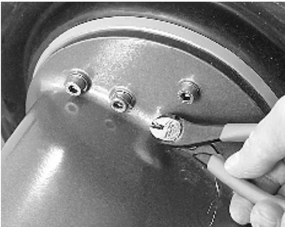
2. Remove the locking wire from the four screws.
