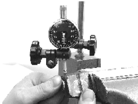
74. Check the clearance between fork and shaft.
