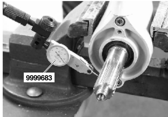
48. When the highest torque specified above has been reached, the gear housing should be removed from the vice and fixed vertically instead. Let the tool remain on the gear housing.
