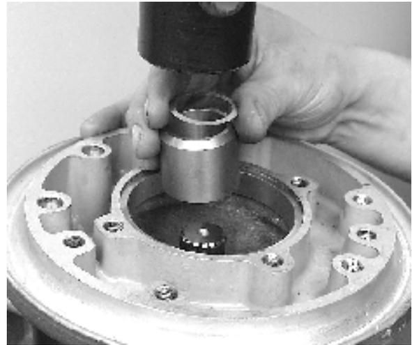
66. Insert the shaft, spacer sleeve and shims with thickness calculated as in item 64.
