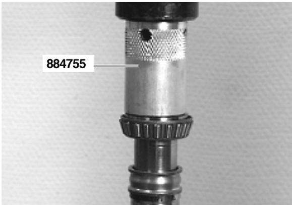
15. Install a new roller bearing with mandrel **884755**.
