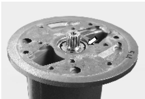
**62.** Install the calculated thickness of shims and gasket on the division plane of the lower gear housing.
